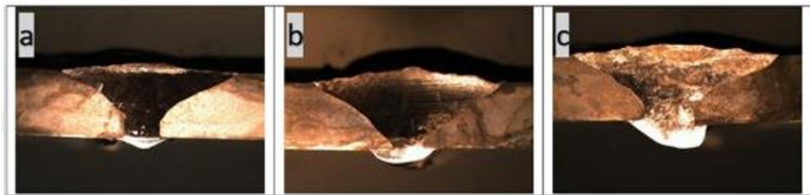
Figure 3. Macrostructure images of the welded joint made with the Citochromax coded electrode (Ø3.25 mm) a) N1, b) N2 and c) N3.
