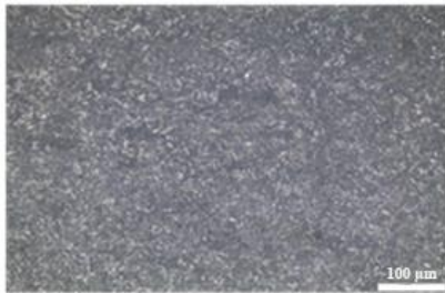
Figure 5. Microstructure images of Miilux Protection 500 base material.
