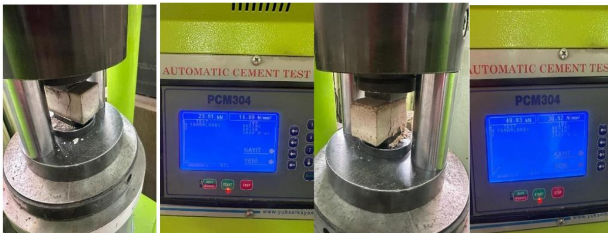
Figure 1. Compressive strength test.
