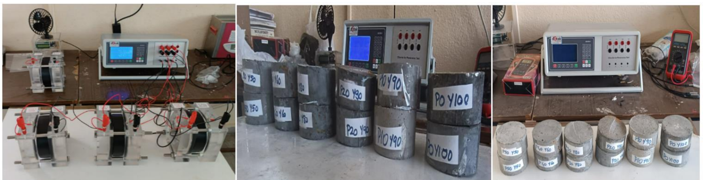
Figure 3. Chlorine permeability of AAS composite mortars.
