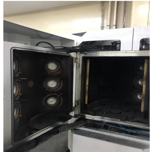
Figure 4. Image of cathode samples used in PVD coating processes.
